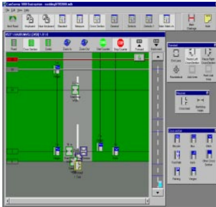
Fig. 2: Screen image of the CamSurvey data collection system showing geometric features positioned along and across the road.
