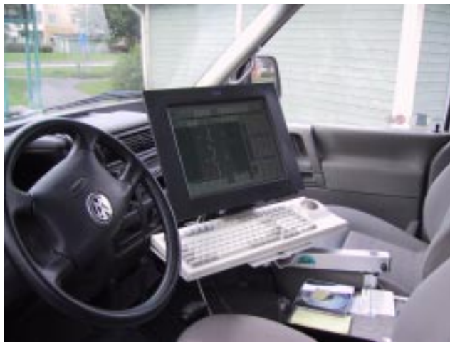
Fig. 1: The touch screen is mounted in the vehicle so that the screen is visible and easily accessible from the driver's seat.
