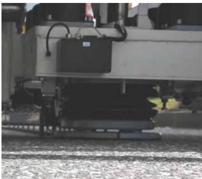
*The four-split load plate allows good contact to the surface and accurate measuring.*
